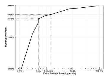
Fig. 8. ROC curve of the parking detection model on the test dataset. The model achieves 99.65% AUC. Two threshold points (0.5 and 0.7) indicated on the curve with their resulting FPR and TPR.
