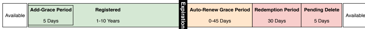
Figure 1: Stages in the life-cycle of a domain name registration. Green or red indicate the domain is present in or absent from the zone files respectively. Orange means the domain may or may not be in the zone files depending on registrar policies.
