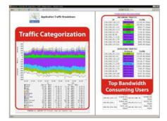
Fig. 1. *AppMon* Web Interface. Traffic classification of the entire network is visualized in the left pane of the interface, while the right pane displays the "heaviest," in terms of network use, IP-application pairs.
