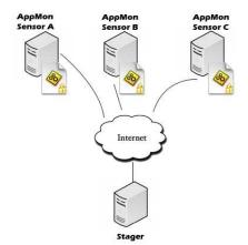
Fig. 4. Step 2: A number of remote *AppMon*-Sensors sending networkmonitoring data securely (encrypted files) to a central *Stager*-Server where our last sub-module will insert them into *Stager*'s database.
